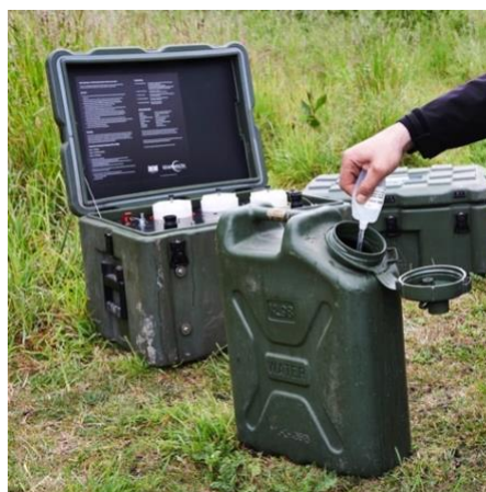
Using ADS to disinfect drinking water in a water can
