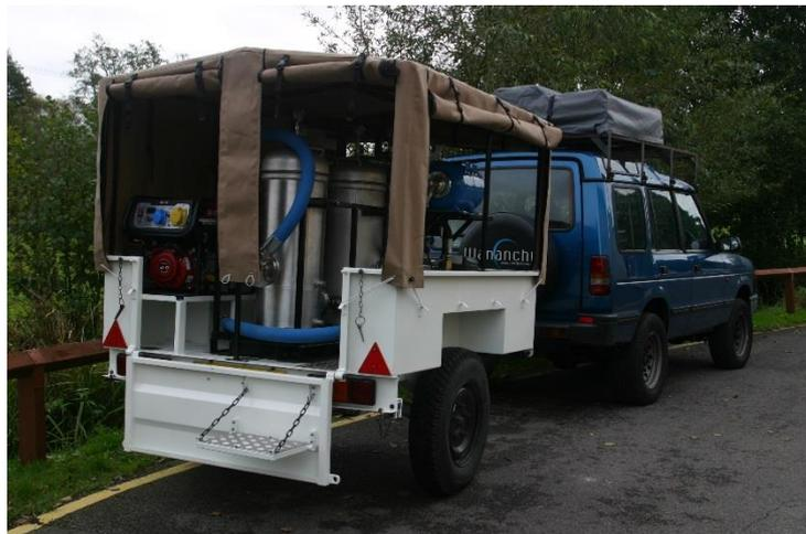
Séon UVT is equipped with multi-stage filtration, Ultra Violet disinfection, integral generator and twin self-priming pumps for full simple on site operation. Chlorine dosing is applied post filtration to ensure bacterially safe water after delivering into end user water vessels of potentially unknown sterility.
