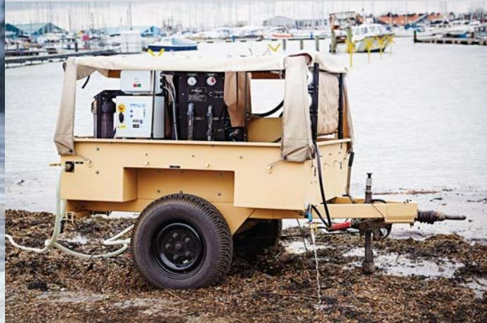
Séon UVT is a bigger, higher capacity version of Séon UV. It uses a similar water purification process with additional chlorine dosing for storage of water. Powered by its on board generator or external power source, it can deliver up to 7200 litres of fresh, safe water per hour.
